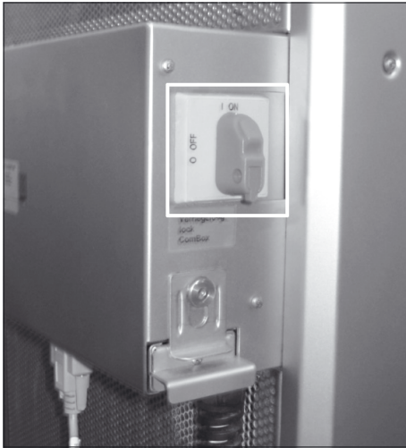
Fig. 9: Cryopilot A Main Power Switch
