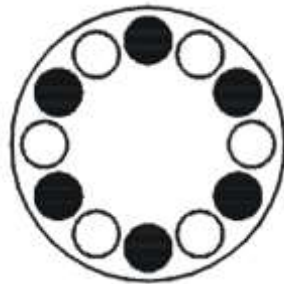
Fig. 4: Permissible and impermissible loading of an angle rotor (example illustration)
