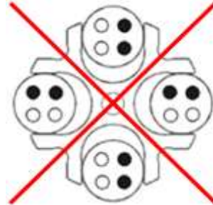
Fig. 6: Permissible and impermissible loading of an angle rotor and a swing-out rotor (example illustrations)
