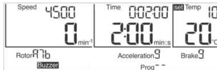
fig. 14: Setting the temperature
