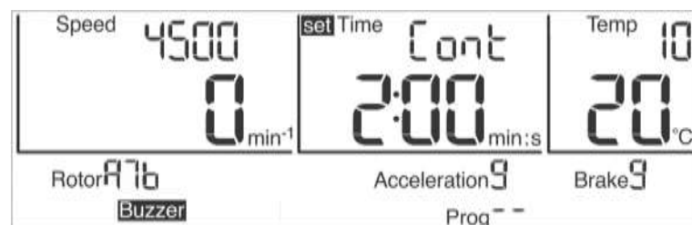
Fig. 12: Indication "Cont" during a continuous run
