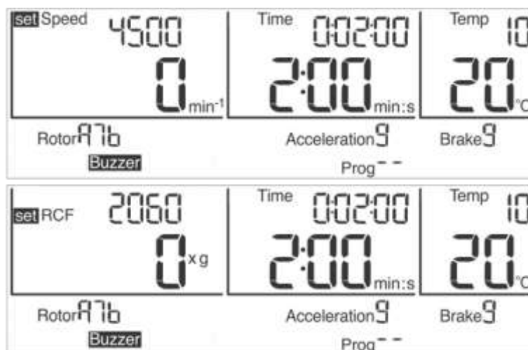
Fig. 9: Setting the speed value or the RCF value
