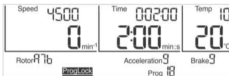
Fig. 20: The program lock "ProgLock" is activated
