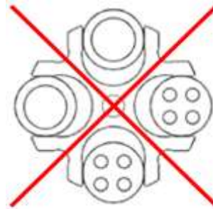
Fig. 5: Permissible and impermissible loading of a swing-out rotor with different tube sizes (example illustrations)
