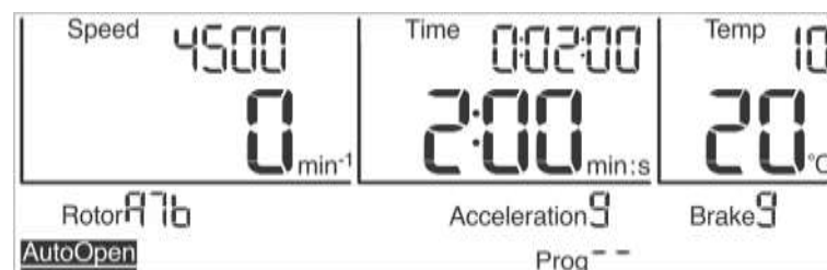
Fig. 18: The automatic lid opening function "Auto Open" is activated
