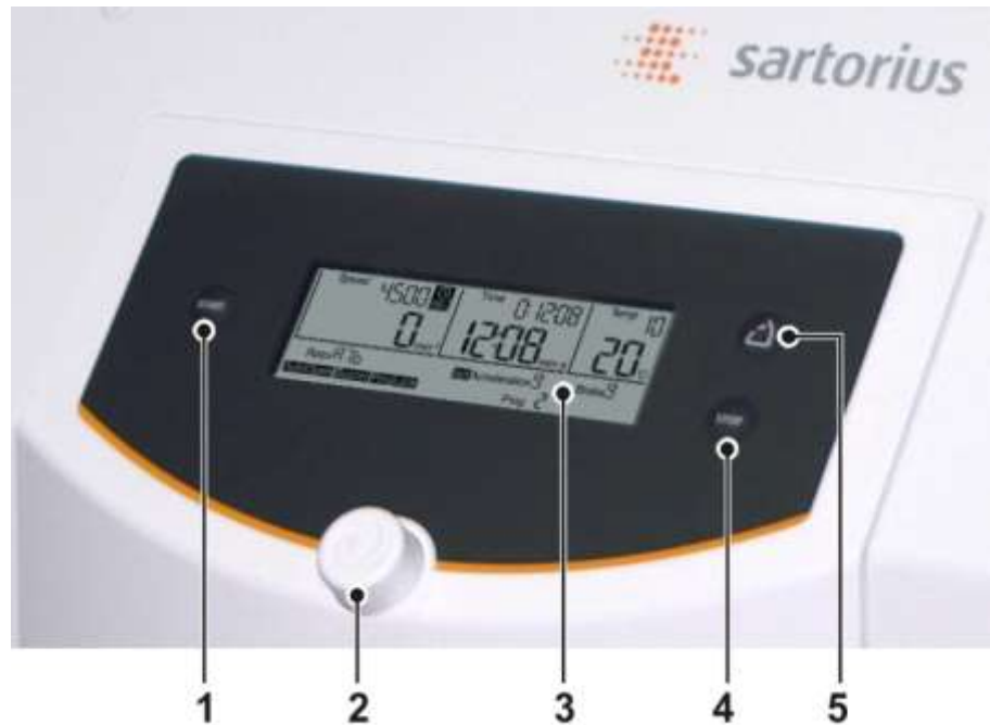
Fig. 7: User interface of the centrifuge
