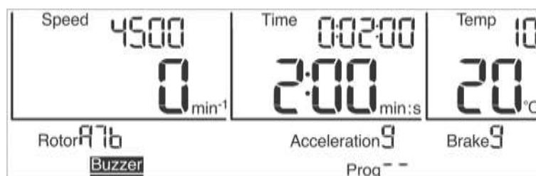
Fig. 19: The sound signal "Buzzer" is activated
