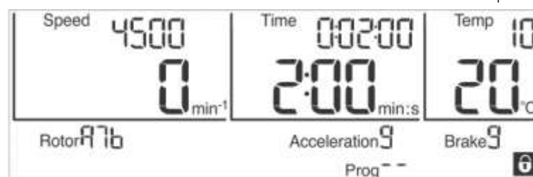
Fig. 23: "Padlock" symbol indicating an activated input lock
