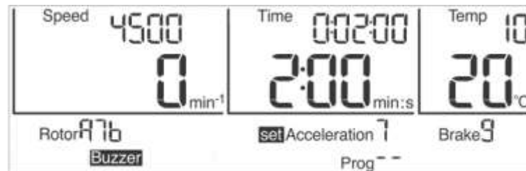
Fig. 17: Preselection of a curve; here: preselection of an acceleration curve
