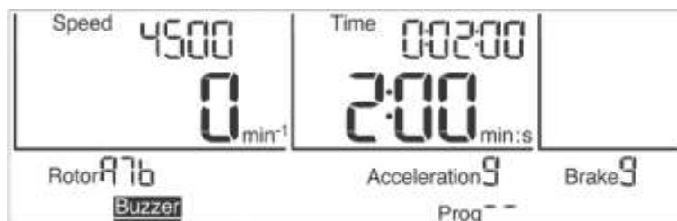
Fig. 18: The sound signal "Buzzer" is activated
