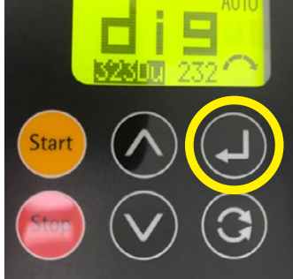
Figure 9: Set pump model 323Du to digital mode
