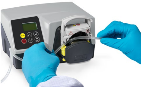
Figure 20: Installing tube in pump head
