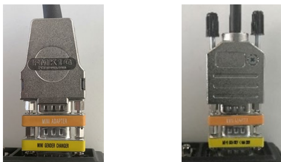
Figure 2: The images show the correct setup at Watson-Marlow 323Du pump using cable YCC04-D25M6 or cable 69Y03295 plus null modem and gender changer.
