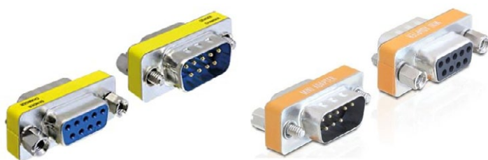
Figure 1: Gender changer and null modem connector for serial cables 69Y03295 or YCC04-D25M6
