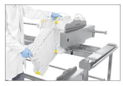
▶ Push the filter down so that the second grip can be reached for an easy handling.
