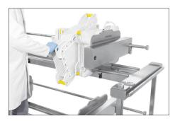
▶ Pull the filter out of the holder until the second groove reaches the first rail.
