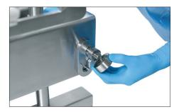
▶ Remove the positioning bars for an easier off-loading of heavy filters.
