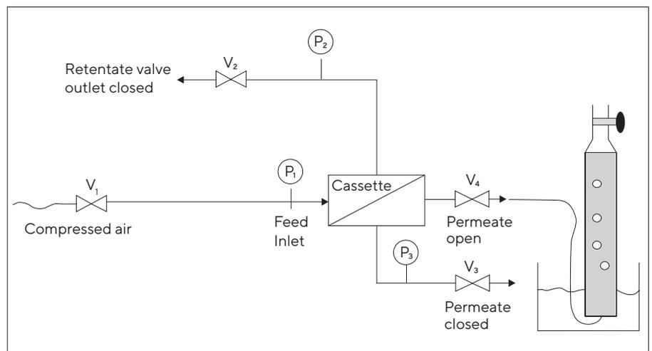
Fig. 13: System set up for manual integrity testing
