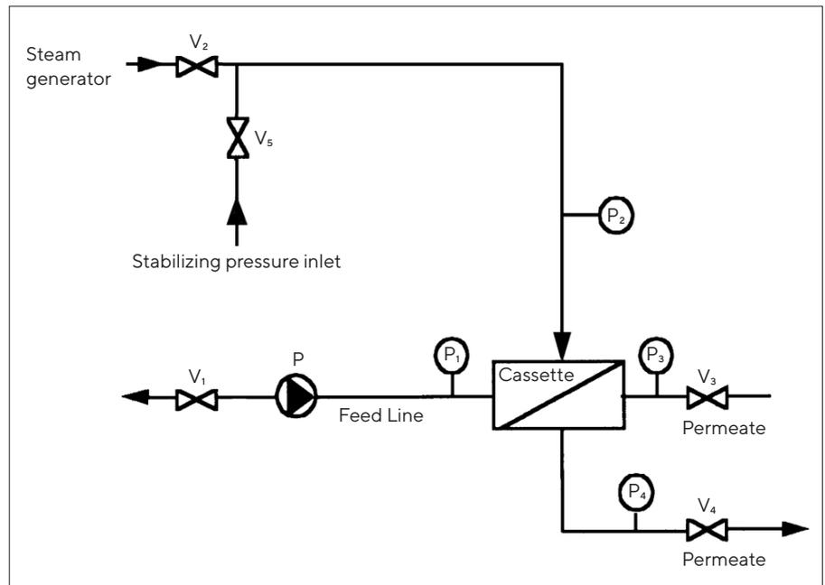
Fig.15: Diagram of the system for in-line steam sterilization of Microfilter cassettes. V<sub>1</sub>-V<sub>5</sub>: valves; P<sub>1</sub>-P<sub>4</sub>: pressure gauge, P: pump
