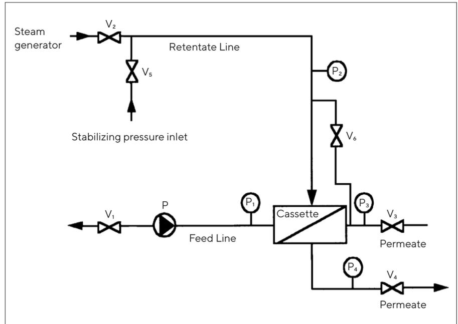
Fig.18: Diagram of the crossflow system for in-line steam sterilization of polyethersulfone Ultrafilter cassettes. V<sub>1</sub>-V<sub>6</sub>: valves; P<sub>1</sub>-P<sub>4</sub>: pressure gauge, P: pump
