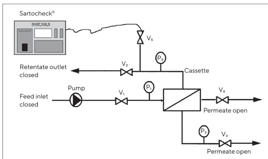
Fig. 14: System set up for automatic integrity testing.  $V_1$ - $V_5$ : valves;  $P_1$ - $P_3$ : pressure gauge.
