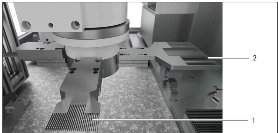
Fig. 10: Portal arm with 1000 gram grippers
