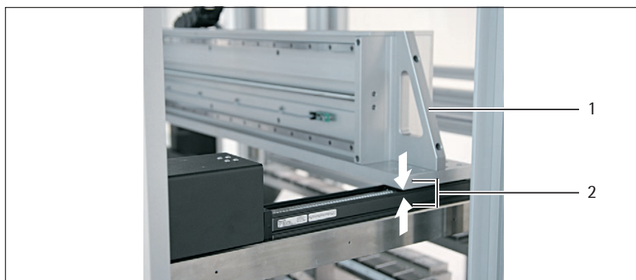
Fig. 17: Position markings for the safety corridor
