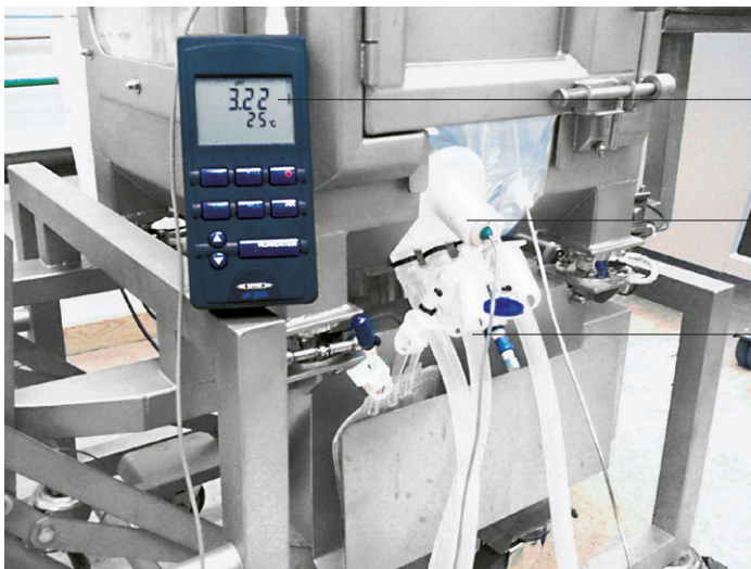
Figure 5: 50 L Flexel® Bag for LevMixer® in 50 L Palletank® for Lev Mixer (weighing)
