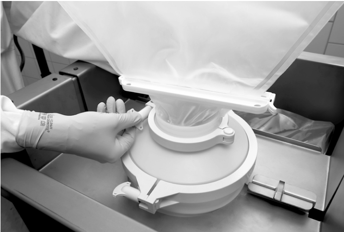
Figure 1: Docking of the 15 L Powder Bag onto the Flexel® Bag for Magnetic Mixer
