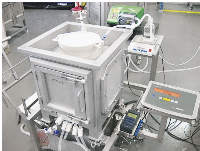
Figure 4: 50 L Flexel® Bag for Lev Mixer in 50 L Palletank® for Lev Mixer (weighing)
