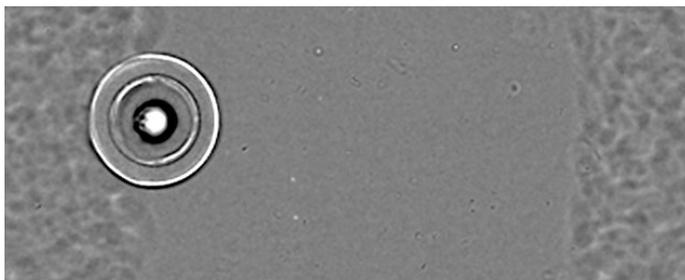
Due to its viscosity, the gel layer of a matrix material may retain bubbles that form during pipetting but would normally escape to the surface. When using Collagen-1,
