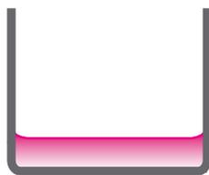
Coat plate surface with 100 mg/mL Matrigel® (50 µL/well) to ensure cell attachment.
