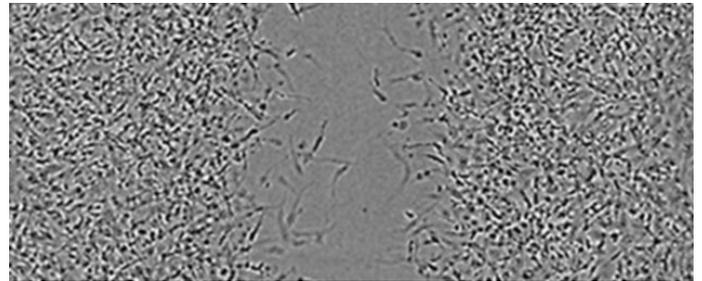
Cells that are plated too densely can lead to the deformation of the biomatrix material, causing cells adhered to it to become out of focus. This can lead to difficulties in image analysis. Careful optimization of cell density can resolve this problem. It is advisable to use the minimum number of cells required to achieve 80–100% confluence at the time of wounding.
