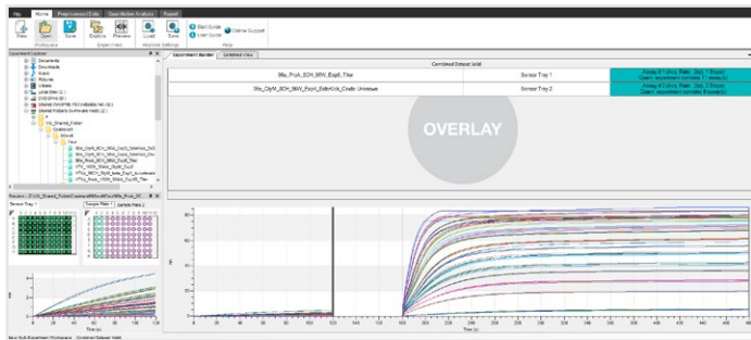
Figure 23: Octet® Analysis Studio Home tab window view. GlyM sensor data and ProA Titer sensor data files can be overlaid together in the software by dragging them into the Experiment Builder window on the right.
