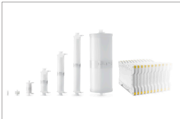
Fig. 1: Sartobind Phenyl capsules: pico (left, 0.08 mL 4 mm bed height) nano 3 mL, 150 mL, 400 mL, 800 mL, 1.2 L, 5 L Jumbo and 1.6 L Cassette (8 mm bed height)
