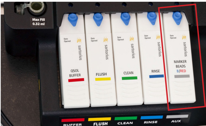
Figure 1. Enhanced Rinse Station. Install a Marker Bead cartridge in the AUX station.
